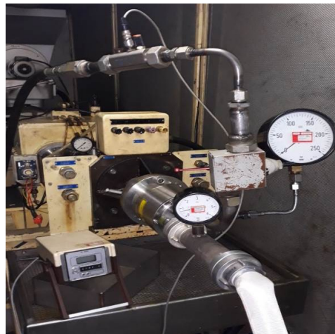
Fig. 3. Water hydraulic axial piston pump installed on the test stand
